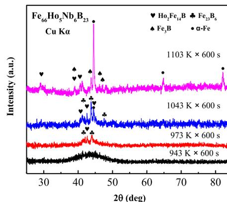
Fig. 2. XRD patterns of  $\text{Fe}_{66}\text{Ho}_5\text{Nb}_6\text{B}_{23}$  ribbons at different annealing temperatures.
