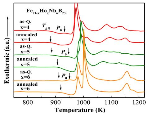
Fig. 5. DSC curves of both as-quenched and isothermally annealed for 120 s of  $\text{Fe}_{71-x}\text{Ho}_x\text{Nb}_6\text{B}_{23}$  ribbons samples ( $x = 4, 5, 6$  at. %).
