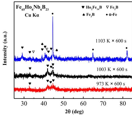
Fig. 3. XRD patterns of  $\text{Fe}_{65}\text{Ho}_6\text{Nb}_6\text{B}_{23}$  ribbons at different annealing temperatures.
