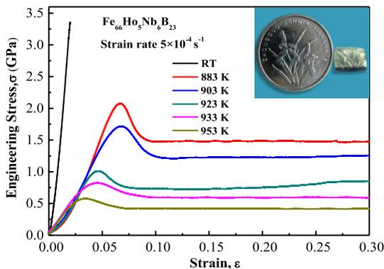
Fig. 8. The compressive stress-strain curves of 1 mm  $\text{Fe}_{66}\text{Ho}_5\text{Nb}_6\text{B}_{23}$  as-cast rods at different temperatures. The inset figure shows the pattern of a Chinese dime coin imprinted into the  $\text{Fe}_{66}\text{Ho}_5\text{Nb}_6\text{B}_{23}$  BMG sheet at 953 K.
