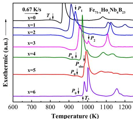
Fig. 1. DSC curves of melt-spun  $\text{Fe}_{71-x}\text{Ho}_x\text{Nb}_6\text{B}_{23}$  ( $0 \leq x \leq 6$ ) glassy ribbons.
