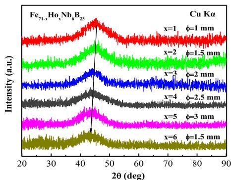
Fig. 4. XRD patterns of  $\text{Fe}_{71-x}\text{Ho}_x\text{Nb}_6\text{B}_{23}$  ( $1 \leq x \leq 6$ ) glassy rods with critical diameters of 1, 1.5, 2, 2.5, 3, and 1.5 mm, respectively.
