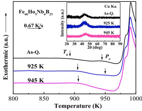
Fig. 6. DSC curves of the  $\text{Fe}_{66}\text{Ho}_5\text{Nb}_6\text{B}_{23}$  samples annealed at various temperatures. The inset figure shows XRD patterns of the annealed samples.
