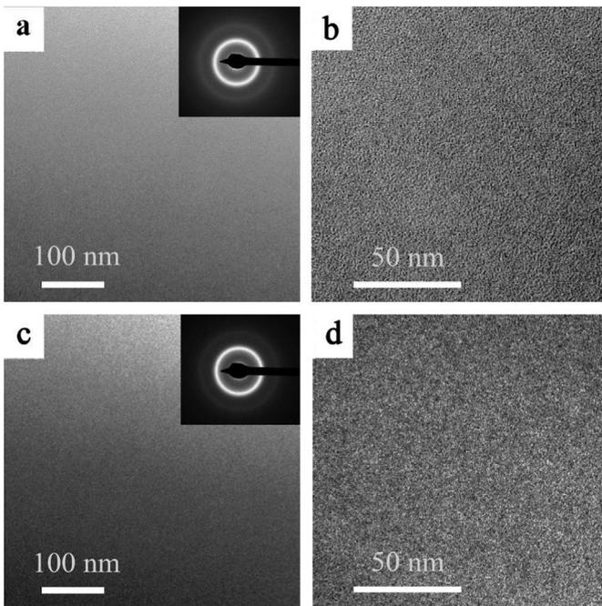
Fig. 7. TEM images obtained from the  $\text{Fe}_{66}\text{Ho}_5\text{Nb}_6\text{B}_{23}$  ribbons in the as-melt spun state: (a) and (b). TEM images of the  $\text{Fe}_{66}\text{Ho}_5\text{Nb}_6\text{B}_{23}$  ribbons once heated up to 945 K: (c) and (d).
