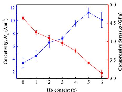
**Fig. 10.** The coercivity (left axis) and compressive stress (right axis) of  $\text{Fe}_{71-x}\text{Ho}_x\text{Nb}_6\text{B}_{23}$  ( $0 \leq x \leq 6$ ) glassy alloys as a function of Ho content.
